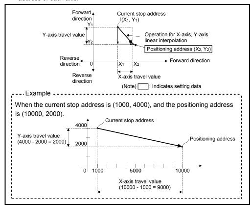
Fig.6.3 Positioning using absolute data method
