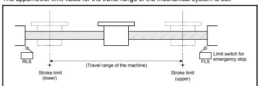
Fig. 4.3 Travel range at the upper/lower stroke limit value setting
