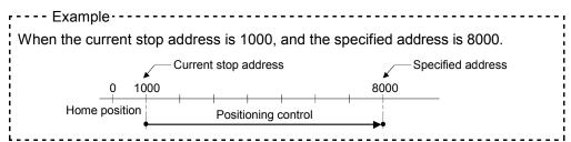
Fig.6.1 Positioning using absolute data method
