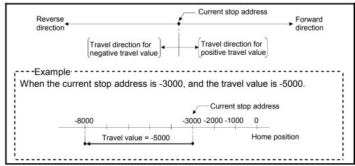
Fig.6.2 Positioning using incremental data method
