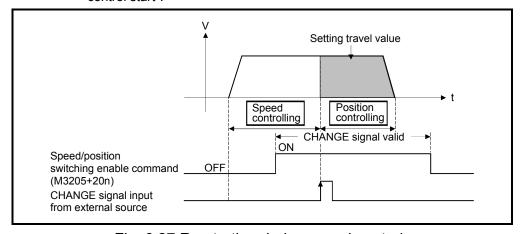
Fig. 6.27 Re-starting during speed control
