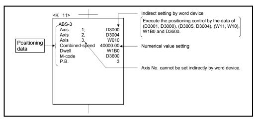
Fig. 5.4 Example of setting positioning data by numerical value setting
