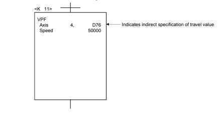
(b) The travel value is stored in the data register for travel value change during speed control in the Motion SFC program. When the CHANGE signal turns on, the contents of the data register for travel value change are set as the travel value.
