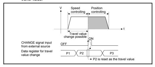
(5) Travel value area after proximity dog ON The travel value since the position mode was selected by the CHANGE signal input from external source is stored in the travel value storage register after proximity dog ON. (Refer to Section 3.2.1)
