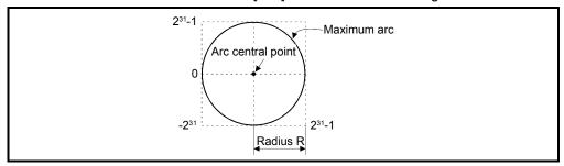
Fig.6.22 Maximum arc radius
