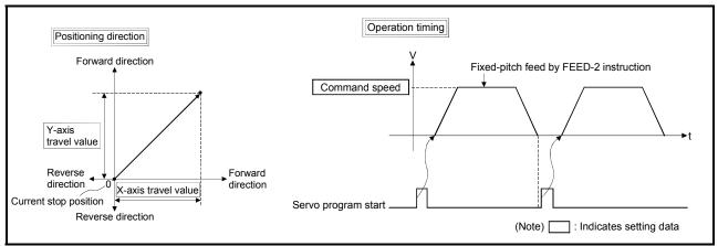
Fig.6.24 Fixed-pitch feed control using 2 axes linear interpolation
