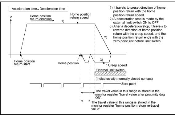
Fig. 6.43 Home position return operation by the limit switch combined type
