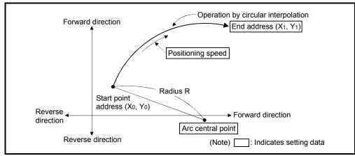
Fig.6.17 Circular interpolation control using absolute date method
