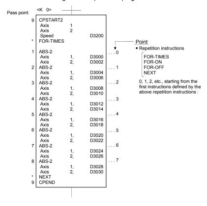
The input situation of positioning data to the Motion CPU is shown the next page by executing the 2-axes constant-speed control using above the servo program and updating the positioning data in indirect devices D3000 to D3006.
