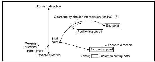
Fig.6.20 Circular interpolation control using incremental data method (INC ? )
