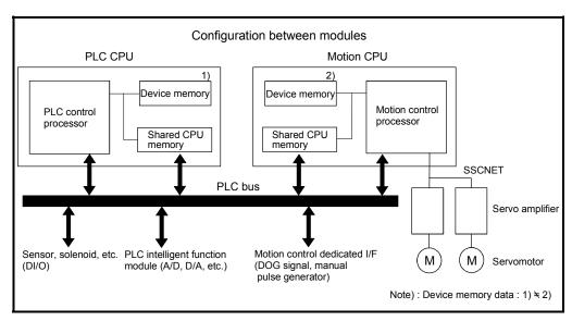
Fig.3.1 Flow of the internal signals/external signals
