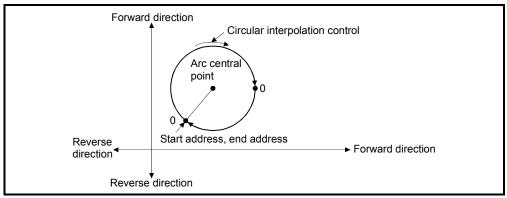
Fig.6.21 Positioning control of a complete round
