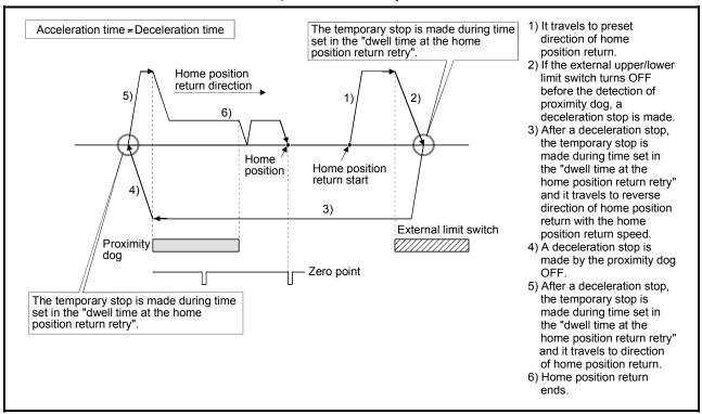
Fig. 6.31 Operation for home position return retry function
