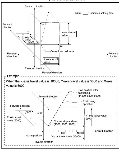
Fig.6.6 Positioning using incremental data method
