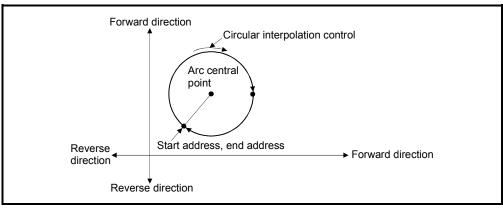
Fig.6.18 Positioning control of a complete round
