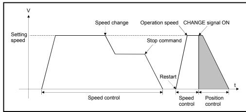
Fig.6.29 Re-starting after speed change
