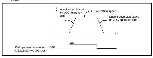
JOG operation for axis for which JOG operation command is turning on is executed.
