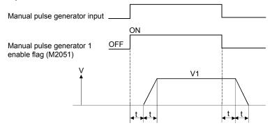
Output speed (V1) = [Number of input pulses/ms]  $\times$  [Manual pulse generator 1- pulse input magnification setting]
