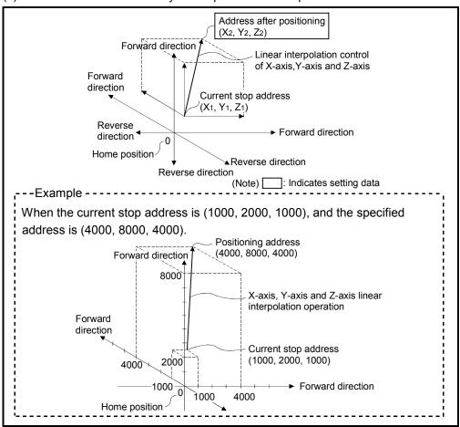
Fig.6.5 Positioning using absolute data method
