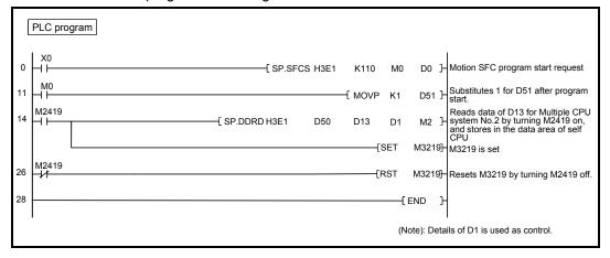
(f) Parameter setting (GSV□P) The CPU shared memory setting example for FIN signal wait function is shown below.
