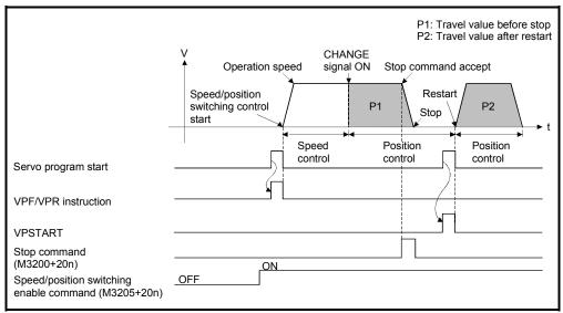
Fig.6.28 Re-starting during speed control
