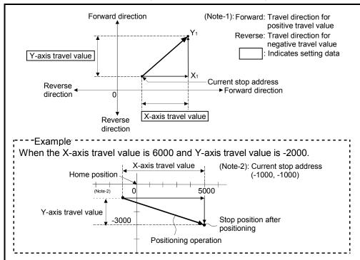
Fig.6.4 Positioning using incremental data method
