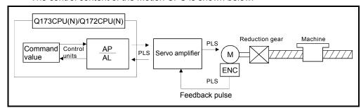
Fig. 4.1 Control content of the Motion CPU
