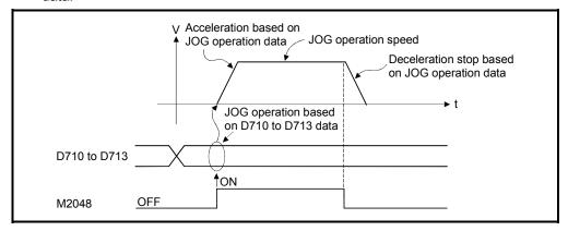
(2) JOG operation axis is set in the JOG operation simultaneous start axis setting register (D710 to D713).
