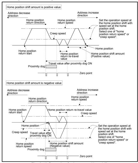
Fig. 6.46 Operation for home position shift
