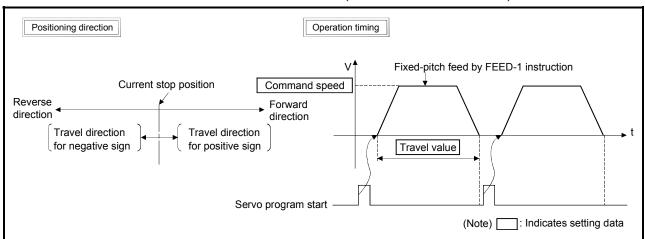
Fig.6.23 1 axis fixed-pitch feed control
